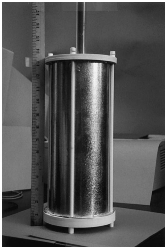
Fig. 9. Photographic picture of our single unit Calvet calorimeter built from an assembly of alumina refractory cylinders in 1965. The photograph was taken after the calorimeter was dismantled in the 1990s.
